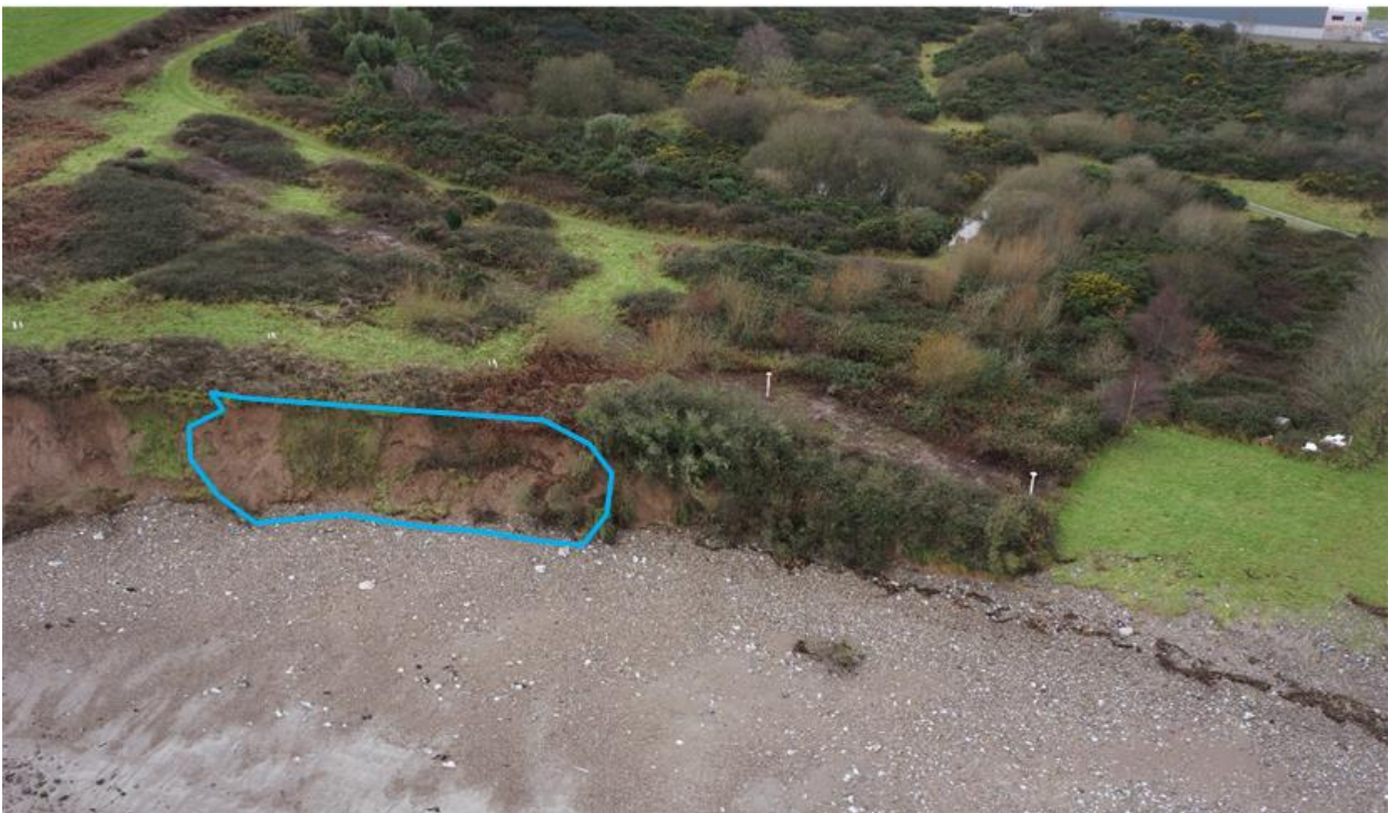
Figure 1 Drone photography showing first area of slope failure and minimal damage to the beach north of this location
